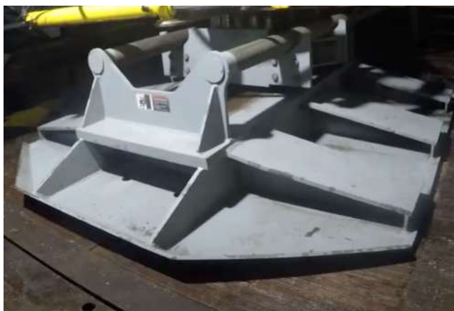
The walking “foot” of H&P FlexRig 269. Source: www.helmerichpayne.com .
