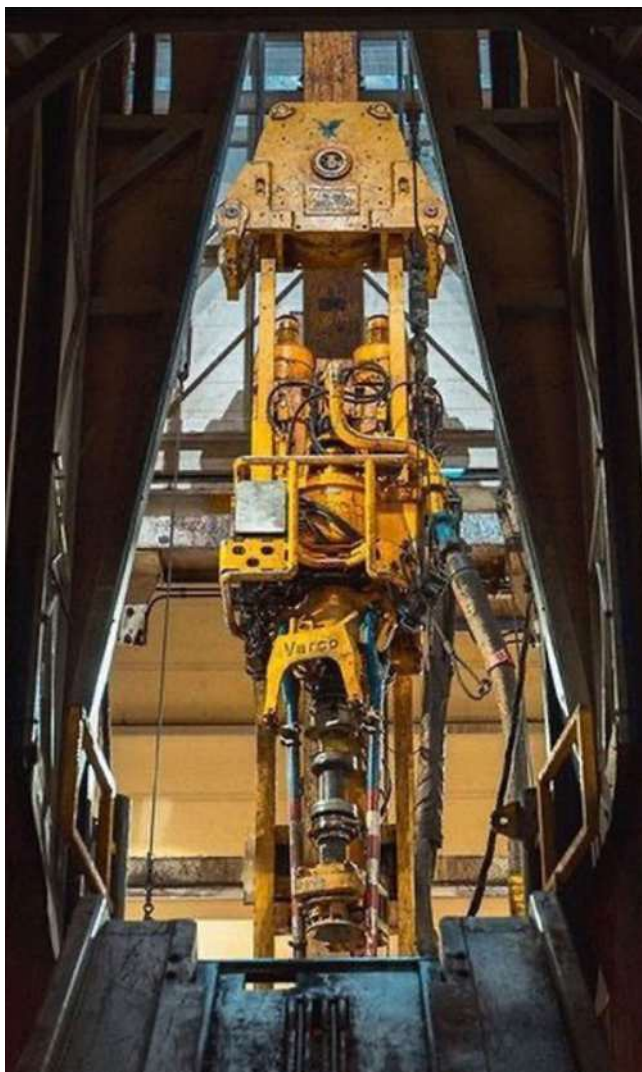
Topdrives were used mainly offshore before the 1990s, when onshore applications opened up a new market and a new way of drilling onshore wells.
